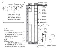
Note The power supply voltage must be 100 to 240 VAC or 24 VAC/DC for the E5ER-T to comply with CE marking requirements. The power supply voltage must be 100 to 120 VAC or 24 VAC/DC for the E5ER-T to comply with UL requirements.
